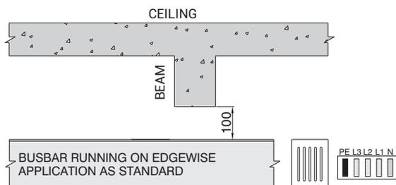
**FIGURE 5 - CROSSING UNDER A BEAM ON FLATWISE APPLICATION**
